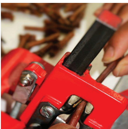
Figure 5. Vine being grafted in V graft machine.
